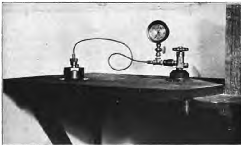
Fig. 11. Filling an Oxygen Bomb from a High-pressure Cylinder Supply (Courtesy of the Standard Calorimeter Co., East Moline, Ill.)
